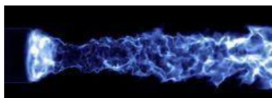
Figure-1 Volume rendering of a non-premixed swirl flame as simulated by LES.
